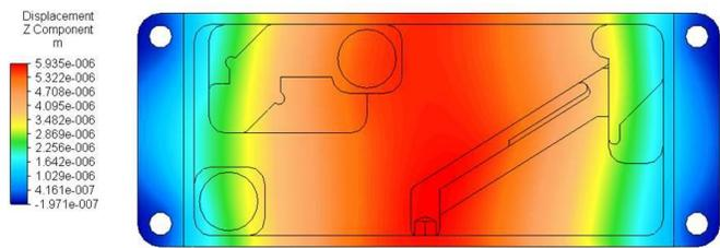
Figure 6: Stiffness analysis of the laser chassis when 50 psi force was exerted on each mounting hole.
