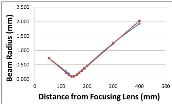
Figure 3:  $M^2$  measurement of the laser beam.  $M^2$  is < 2 in both axis.
