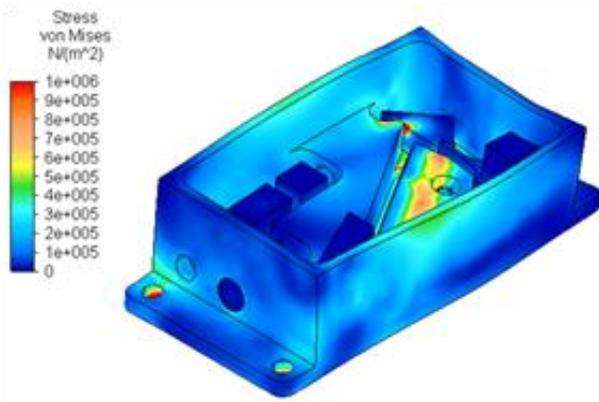
Figure 9: Stress in the laser chassis when subjected to random vibration of 14 Grms. Maximum stress is 1 MPa which is orders of magnitude below the tensile strength of CuW.
