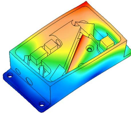
Figure 10: Modal analysis of the laser package. First mode is at 3 kHz.
