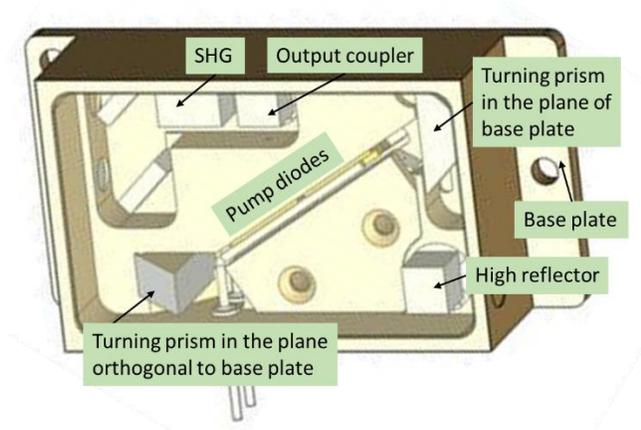
Figure 7: Improved laser chassis design. Dimensions are  $67 \times 32 \times 18$  mm.
