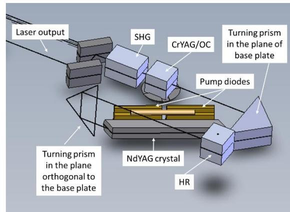
Figure 8: Optical layout of the laser.
