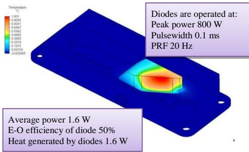
Figure 5: Heat distribution in the laser chassis.
