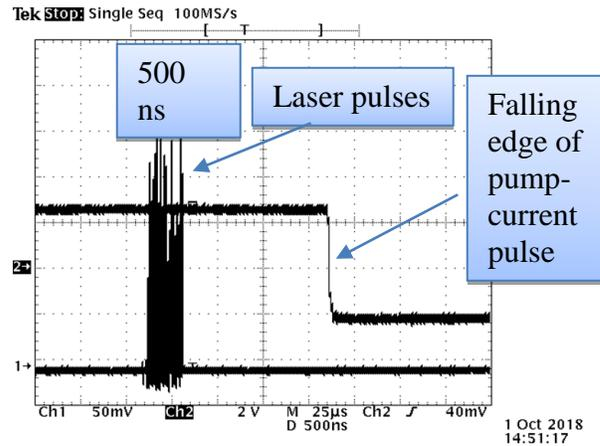
Figure 4: Pulse-to-pulse timing jitter is < 1  $\mu$ s. Scale is 500 ns/div. Accumulation of 256 pulses.
