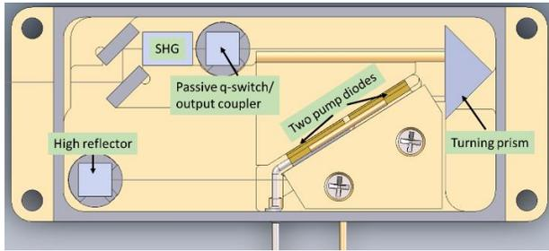
Figure 1: A top view of CAD model of the laser. Resonator was folded using a turning prism for compactness. Dimensions are 80×32×9 mm in L×W×H.
