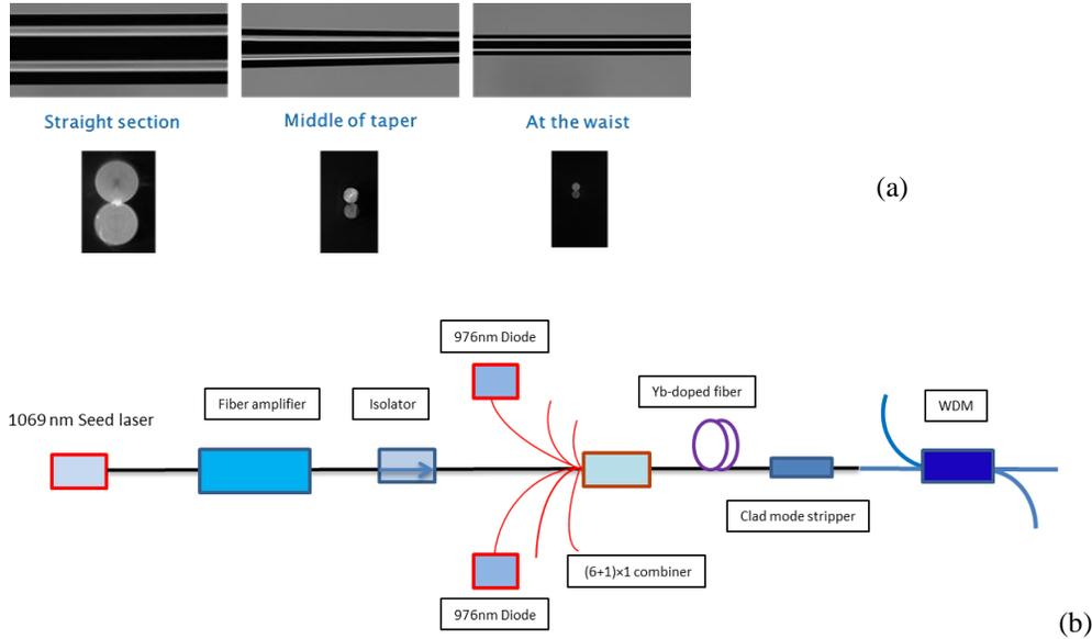
Fig. 2. (a) WDM pictures taken by the high resolution camera on the glass processing machine, (b) schematic of high power laser at 1069 nm.
