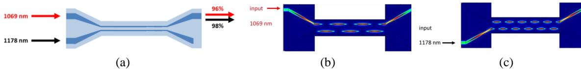
Fig. 1. (a) Modeling structure of a WDM that has straight, tapered, and waist sections (b) & (c) energy transfer between two fibers at 1069 nm and 1178 nm respectively.
