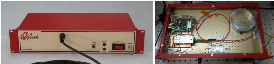
Figure 6. CW Tm: fiber laser provides up to 10 W of single-mode output at 2050 nm.
