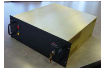
The dimensions of the Q-Peak MPL controller is 20"(L) x 17"(W) x 7"(H).
