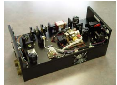
The dimensions of the laser head are 20"(L) x 10"(W) x 8"(H).
